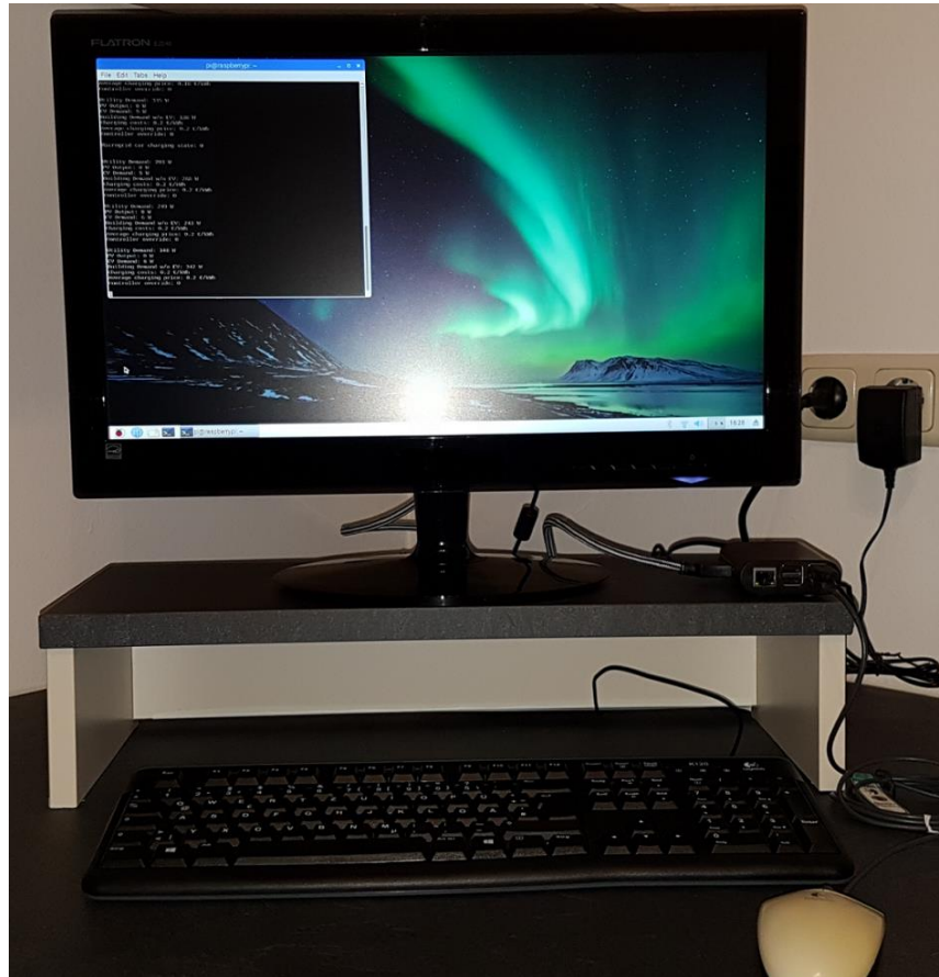
Figure 3: Operational wireless enabled Raspberry Pi controller (small black box on the right) with the controller modules running (small window on the screen).
