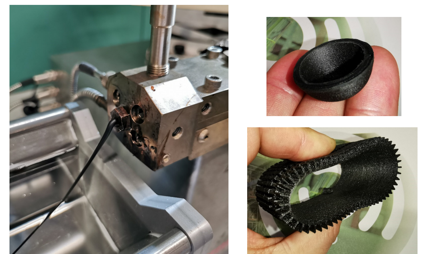
Fig.2 : Compounding tests, production of composite filaments and samples of 3D-printed polymer composites .
