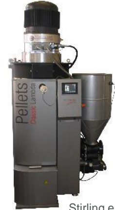
Stirling engine in pellet boiler
