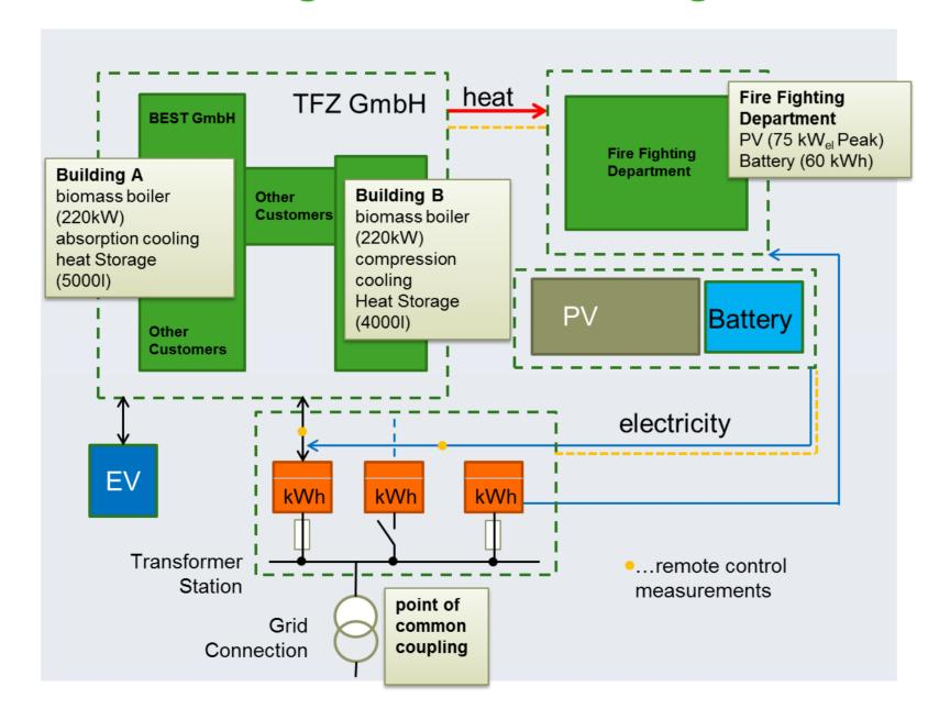
fig. 2) Concept of Microgrid Lab Wieselburg
